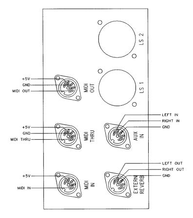
At the rear of the console (seen from the rearside at the very right, in the middle) several DIN connectors are located (see above drawing). The functions of these connectors are the following:
